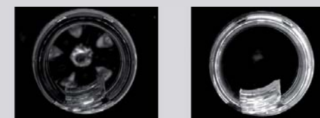
Object: Plastic bottle. Defect on top of a plastic bottle is clearly identified.
