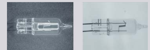
Object: Light bulb. Resulting image clearly shows silhouette of filament inside the bulb.
