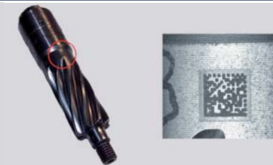
Object: Data Matrix on a gear shaft. Diffuse illumination allows clear image capture of marked symbol.
