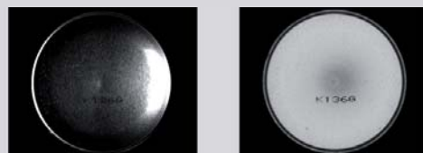
Object: Bottom of aerosol can. Uniform illumination of concave surface results in contrast against printed characters.
